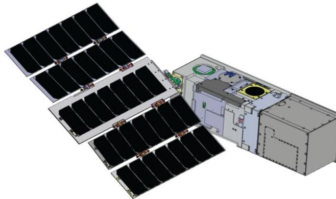
**Figure 6:** The TROPICS space vehicle showing CubeSat bus, radiometer payload, and deployed articulated solar array (Blackwell et al., 2018).
